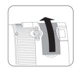
2. Insert the battery into the battery compartment according to the negative and positive directions as illustrated in the picture. Push the battery down until it locks in place.
